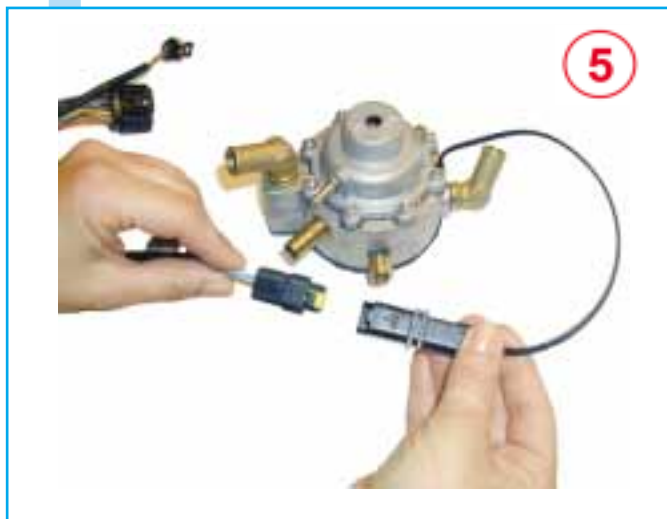
Figure 5: Installation of the temperature sensor (LPG / METHANE).
