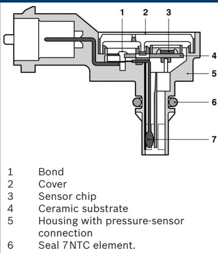
**Section through sensor cell**
