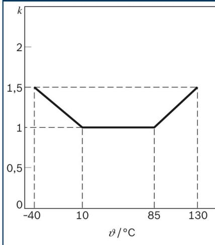
**Characteristic curve for temperature sensor**
