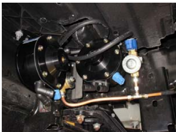
Mount LPG-piping with T-piece to reducers. Solder 2 nd reducer plug to cable-wiring.
