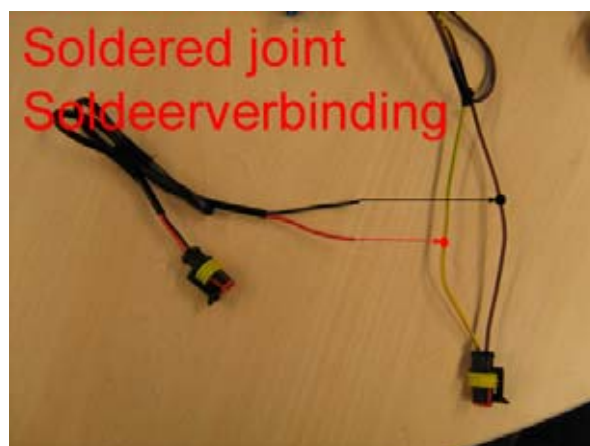
Mount LPG-piping with T-piece to reducers. Solder 2 nd reducer plug to cable-wiring.
