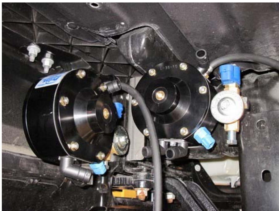
Mount Ø5mm overpressure hose to reducers. Mount the reducers on the brackets with M8 nuts and springwashers.
