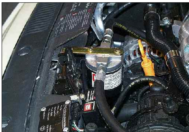
Picture 08 “FJ1” gaseous phase filter
