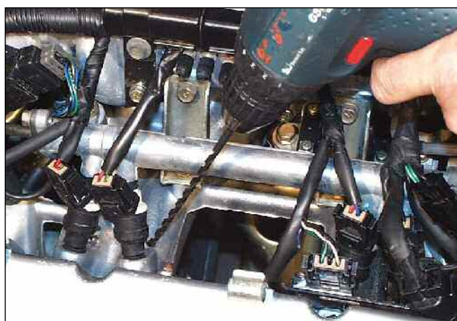
Picture 23 Drilling of manifold
