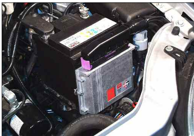
Picture 29 ECU installation in the engine compartment
