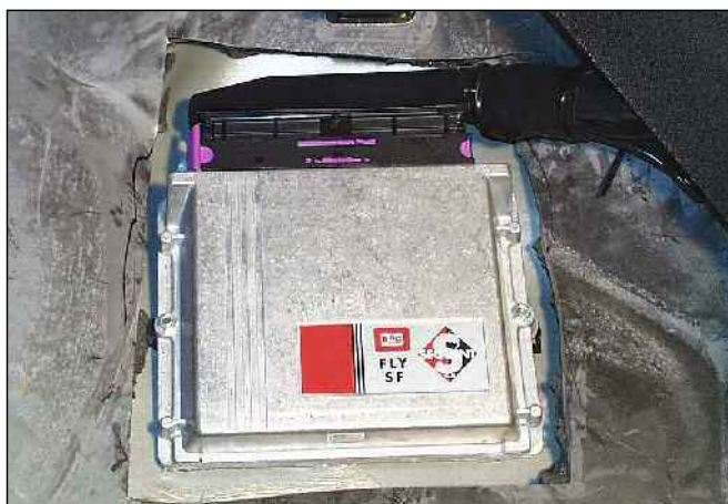
Picture 28 ECU installation inside passenger compartment
