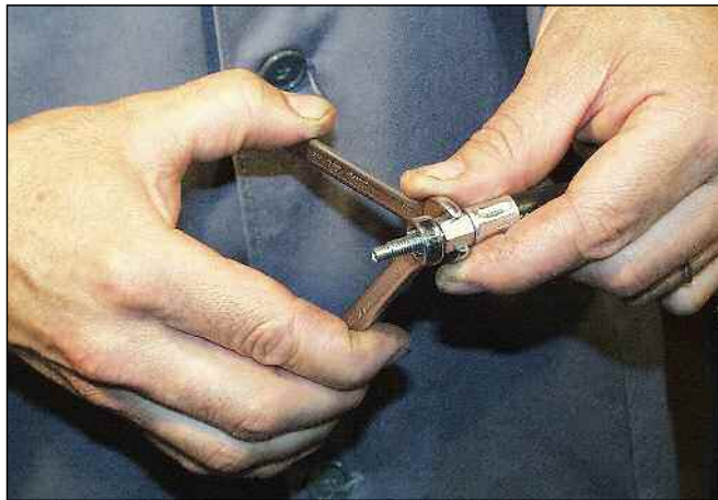
Picture 25 Nozzle clamping on pipe-fitting Solo per injectors BRC
