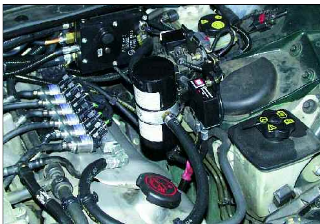
Picture 09 “FJ1 TWIN” gaseous phase filter
