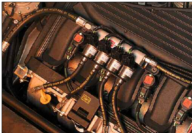
Picture 15 Example of the rail installation with Keihin injectors
