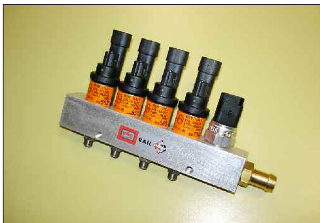
Picture 18 Version with BRC injectors, pressure and gas temperature sensor and rubber-holder connection for Sequent Fastness Applications.
