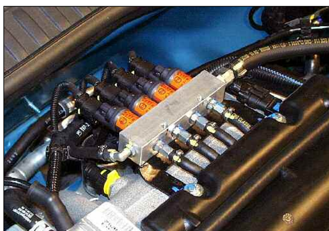
Picture 14 Example of the rail installation with BRC injectors
