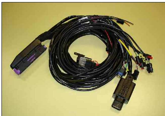
Picture 39 Fly SF ECU main harness for Sequent Fastness applications
