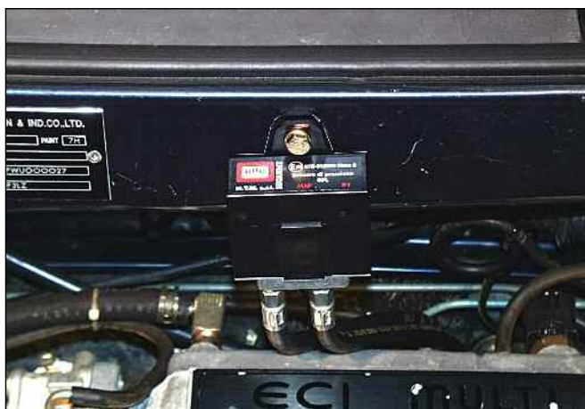
Picture 16 Example of the P1-Map sensor installation
