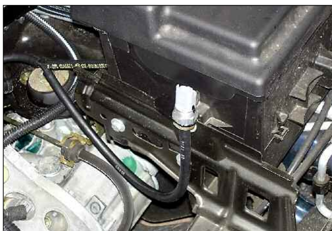
Picture 17 Example of the Sequent Fastness MAP sensor installation
