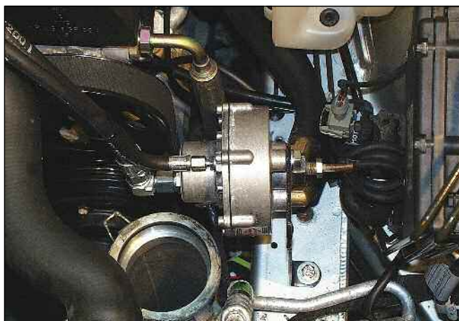
Picture 01 Sequent Genius reducer installation with diaphragm parallel to the driving direction
