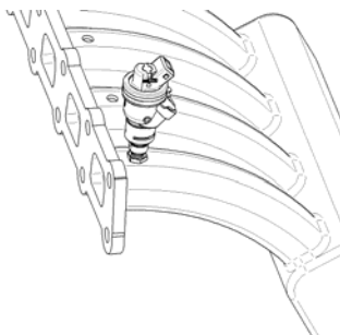
Direct Injector Placing
