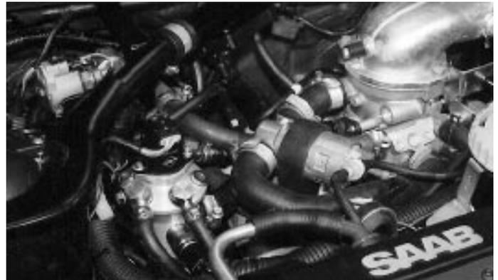
12. *When driving on LPG, the lambda signal to the ECU must be cut and connected to the simulator at the same time. Cut the green wire on pos.23 in the connector on the ECU and attach the red wire coming from the cable harness (lambda-signal) on the sensor side and the red/white wire (simulation) on the ECU-side of the green wire. Connect the 4-way connector to the lambda-simulator 238002-020. Fit the simulator to the heater-housing using a suitable M6 fixing bolt.*
