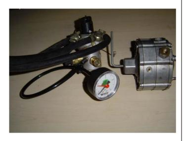
For assembling the gas output tube, we have to remove the 2 short bolts beside the hole.
