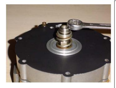
The next we lay on is the big aluminium disk followed by the spring, aluminium ring with the groove for the security ring and the security ring.
