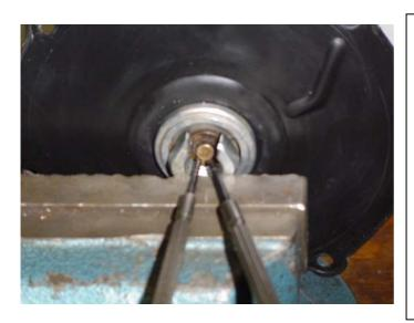
For separating the escort shaft from the membrane of the first step pressure regulator we use a M10 nut where we saw out a little part like is shown on this picture.
