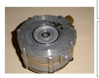
The front side we can close now with the front cover and fix this evenly with the 5 long bolts.(M5x40)
