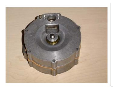
The next part is the vaporisers chamber with in it the second step pressure regulator.
