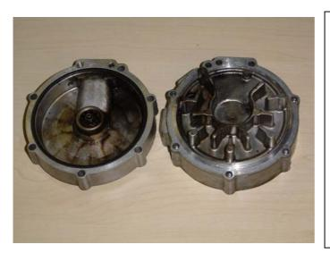
The next step is separating the three parts in the middle op the vaporiser.
