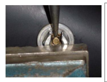
For assembly the escort shaft in the membrane of the first step pressure regulator we use the M10 nut.
