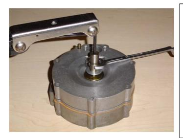
On the second step pressure regulator we fix now the steel shaft with a fork spanner and the inside spanner.
