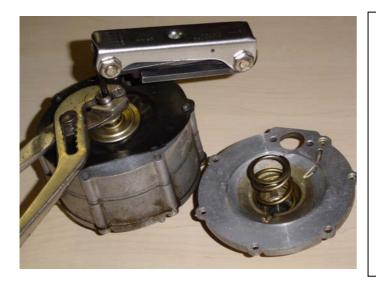
For turning of the steel shaft we need a pair of pliers and an inside spanner.
